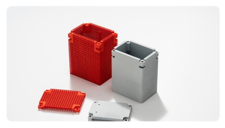
The ability to design complex topologies in 3D printing is a significant advantage that allows you to optimize the structure and performance of printed elements. Traditional manufacturing methods are often limited by standard forms and geometries, which can lead to material waste and poor mechanical properties. Topology in 3D printing introduces a revolutionary approach to design where structure and material are tailored to specific loads and applications.
